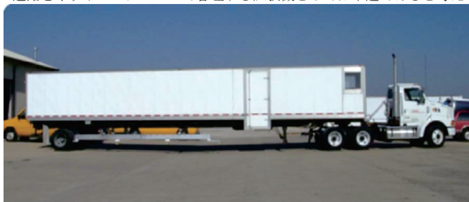
写真-1 RWD (Rolling Wheel Deflectometer (米国)) 13)
