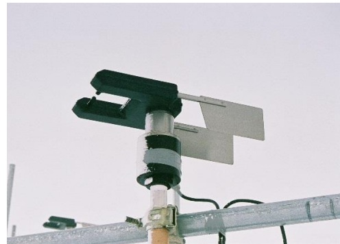
図9 Snow Particle Counter (SPC)の外観
