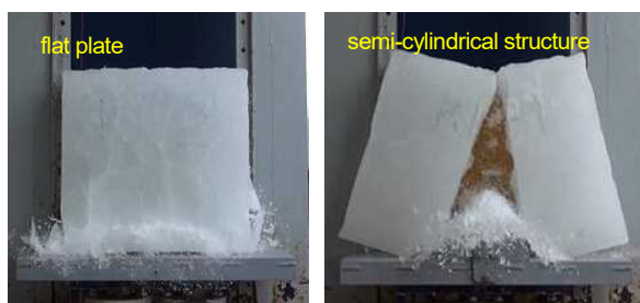
Failure patterns of ice mass with flat plate and semi-cylindrical structure
