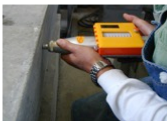
Figure 4: Measurement of rebound number
