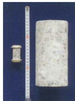
Figure 7: Comparison of a small diameter core (diameter of 25mm) and a standard core (diameter of 100mm)
