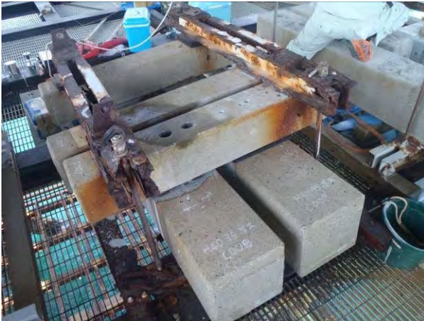
写真-資 3.8 暴露状況 (C002, C003, C004, C007, C008)
