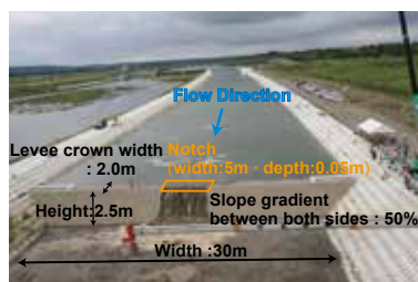
Technical evaluation using full-scale experiment
