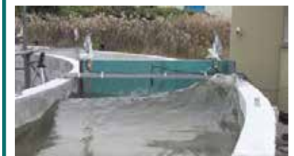
Understanding the effect on structures by experiment of tsunami running up a river
