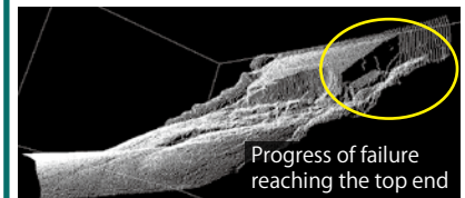
Progress of failure verified by the permeation model experiment
