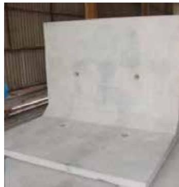
L-shaped retaining wall using recycled aggregate (provided by Prof. M. Kitatsuji, Miyagi University)
