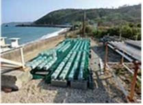
Outdoor exposure tests of concrete specimens
