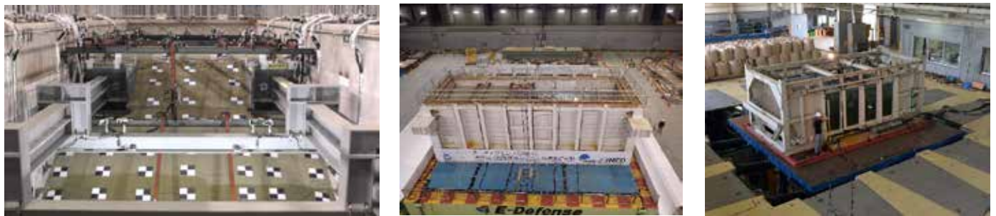
Liquefaction experiment conditions. Left: appearance after the experience using the E-Defense simulator. Vibrations caused cracks in the earth bank. Middle: the E-Defense experiment conditions as used in the latest experiment. Right: PWRI experiment conditions as used in past experiments. The middle and right photographs show investigation of the behavior during an earthquake of an earth bank formed inside the box. The size of the people in the photographs shows the scale of the experiment facilities.
