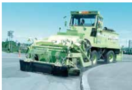
Road surface cleaning by attachment-type road sweeping device for rotary snowplow
