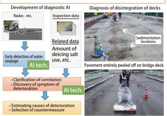
Measurement using radar before peeling the asphalt pavement
