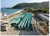
Outdoor exposure tests of concrete specimens
