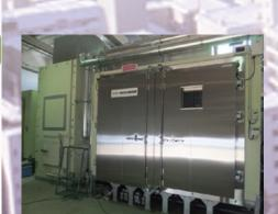
Concrete combined-deterioration accelerating test apparatus
