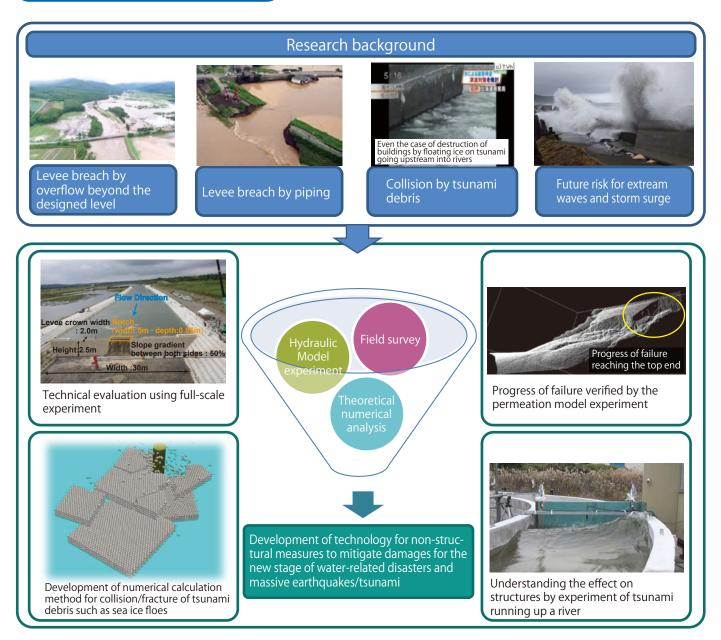
In recent years, intensive and heavy rainfalls in local areas cause frequent floods that is beyond the capacity of facilities. Levees are destroyed by overflow and seepage, and river structures are damaged by high-speed flow. In addition, due to the 2011 Great East Japan Earthquake, working on tsunami disasters has become an urgent issue.
