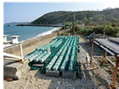
Outdoor exposure tests of concrete specimens
