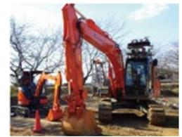
Remotely operated excavator
