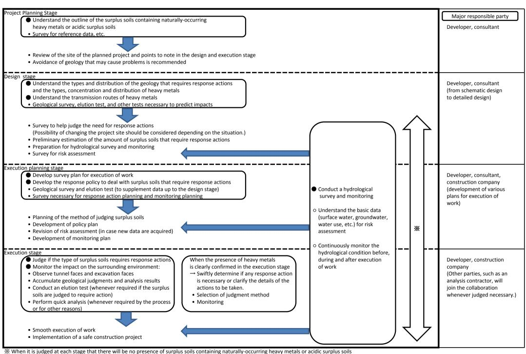
When it is judged at each stage that there will be no presence of surplus soils containing naturally-occurring heavy metals or acidic surplus soil (in case excavated rocks and soils are used for fill, the conditions of the fill location should be considered when making this judgment), it is permissible to omit further surveys and execute the work in an ordinary way without taking any measures during the execution stage.
