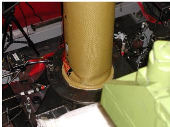
Figure 4. Failure of Steel Pipe Column Wrapped with an Aramid Fiber Reinforced Plastic Sheet.
