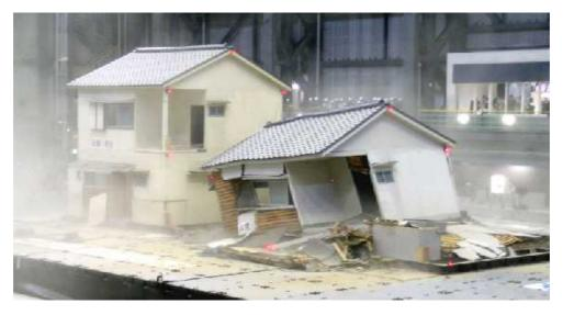
Photo 2. Shake Table Test by E-Defense (Left: Retrofitted, Right: 'As-built')
