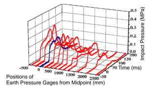
Fig.2: Example of Distribution of Impact Pressure on the Arch
