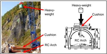
Fig.1: Heavy-weight-falling Experiment for RC Arch
