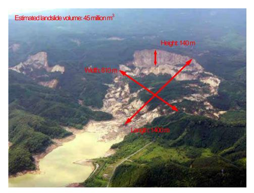
Figure 1. Landslide at Aratozawa
