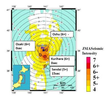
Figure 1: Arcs represent elapsed time (in seconds) from EEW to S wave arrival for Iwate-Miyagi Nairiku Earthquake on 14 June 2008 (M7.2). The differences of color show the observed seismic intensity on JMA scale.
