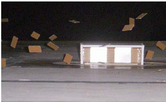
Figure 3. Debris Models Flying around Building Model
