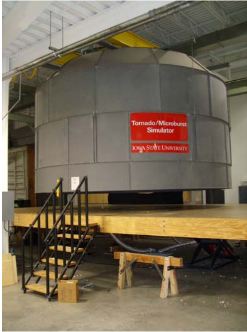
Figure 1. ISU Tornado Simulator
