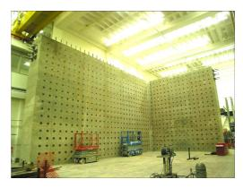
Figure 8. NEES MUST-SIM Reaction Wall (Image courtesy of University of Illinois)
