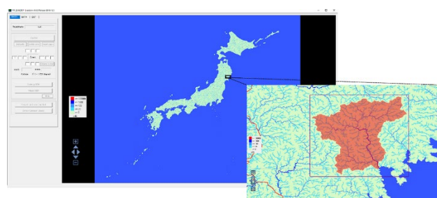
Figure 3-5 RRI-GUI showing the surface flow direction map of Japan and a river basin image extracted from the map
