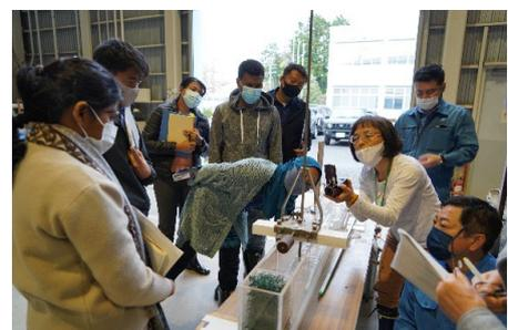
Hydraulic model experiment (Verifying what the student learned in the hydraulics class in the experimental waterway)
