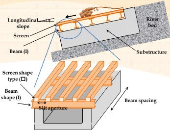
Structure of a debris-flow dewatering brake
