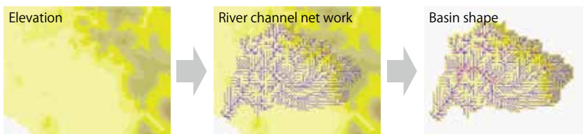
Figure 1 Creation of basin boundary and river channel network on the basis of elevation (The red-framed cells indicate elevation modification.)
