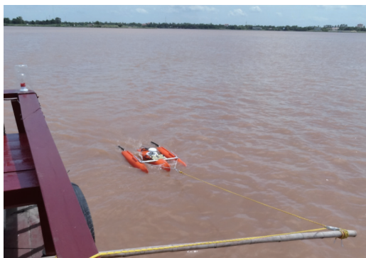
Discharge observation using an aDcp
