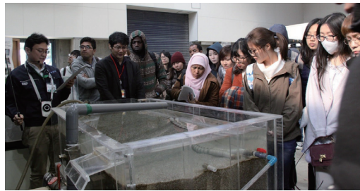
Experiment on removing deposited sediment from a reservoir
