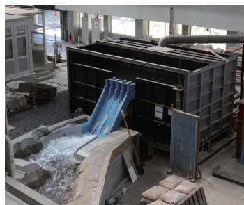
Experiment on a dam spillway
