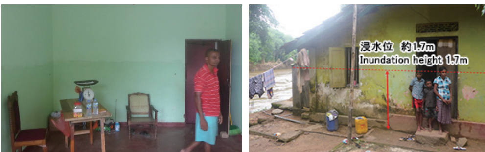
Fig. 5 Field survey of flood levels in the affected areas with guidance of Irrigation department and the embassy of Japan in Sri Lanka
