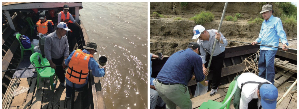
Figure 2: Collection of sediment material from the riverbed and bank for analysis of grain size distribution and sediment properties
