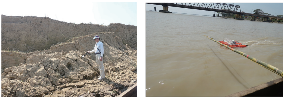
Fig. 3 Collection of bank material (left) and measurement of flow depth and velocity by ADCP (right)
