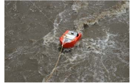
An improved ADCP-mounted radio controlled boat in a field test during flooding
