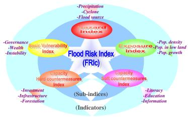
Fig.2 Structure of Flood Risk Index (FRIc)
