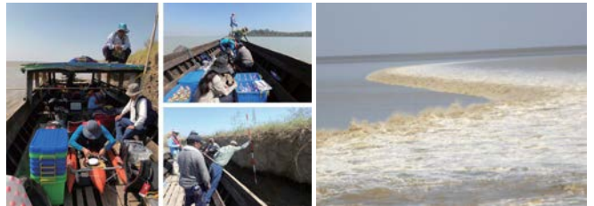
Field investigation in February 2019 in the Sittaung River, Myanmar: preparation of equipment (right), sampling of river water and bank and riverbed material (middle), and a tidal bore in the river estuary. Bank retreat occurs at the rate of 1,000 m/year in some sections where the retreat is most active. The bank erosion is causing life-threatening issues, such as losses of agricultural land and settlements.
