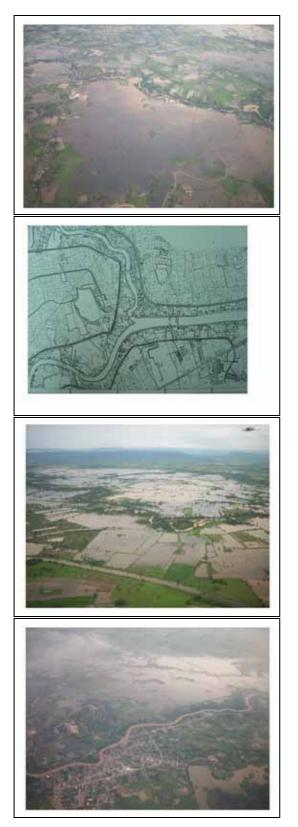
I recently took this aerial image to show the water drainage problems and water logging in the fields. We can see rainwater in the fields and a high water level in the river, both shown in different colors. Therefore, we must urgently improve the drainage system. Highways and houses are located along the river.
