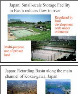
Flooding in 1986 160ha 5 million m<sup>3</sup> capacity Relocated 109 houses Easement agreement with land owners under the legal master plan
