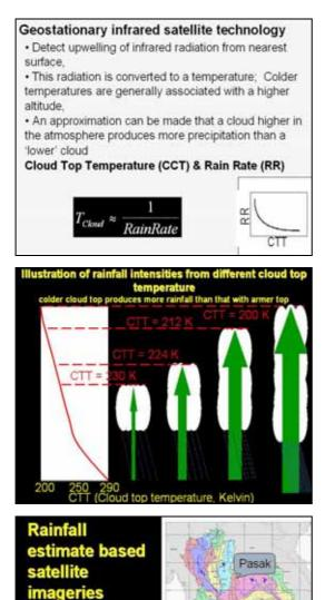
Geostationary infrared satellite technology detects the increase in infrared radiation from the nearest surface. This radiation is converted to temperature: colder temperatures are associated with higher altitudes, which is clear from the connection between the cloud top temperature and the rate.
