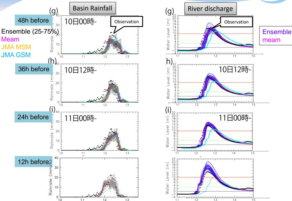
Dam water level operation simulation by using inflow forecastarm
