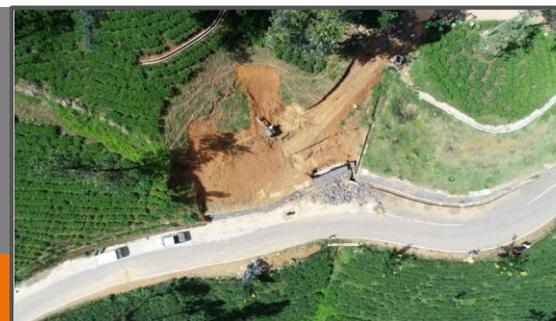
Aerial Photographs obtained from drone surveys are used to generate the contour profiles of sloping terrains
