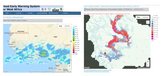
GSMaP real-time visualization (left) and expected maximum inundation depths at hot spots (right) on the FEWS
