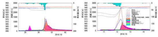
Results of dam operation during the flood caused by a typhoon at Hatanagi Daiiti Dam (left: September 30 to October 1, 2018, right: October 12-13, 2019)
