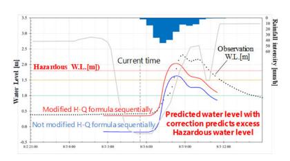
Comparison example of predicted water level with and without H-Q curve sequential correction
