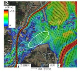
The results of flood flow computation in the Gofukuya River (The color counters show flow depths at the peak discharge.)
