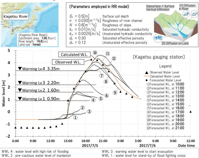
Forecasted flood water levels at specified times using the RRI model with analyzed and forecasted rainfall data. The forecasting used rainfall data forecasted and analyzed by JMA and water stage data from the MLIT water information system. Flow discharge was converted into water level based on the cross-sectional data collected in 2012. 1) Takahiro SAYAMA, Rainfall-Runoff-Inundation(RRI) Model ver. 1.4.2, ICHARM, PWRI (http://www.icharm.pwri.go.jp/research/rri/rri\_top.html)
