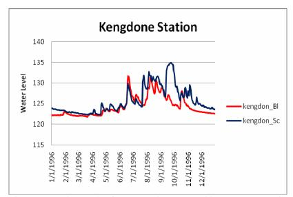
Figure 7: Hydrograph of ISIS result compared between Base Line & Scenario @ Kengdone
