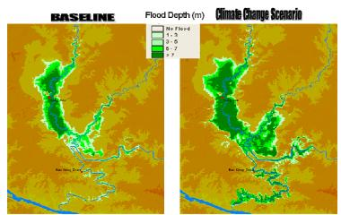
Figure 10: Map of flood depth comparison between base line condition & climate change scenario
