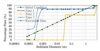
Fig. 13 Temporal Changes of Particle Size Distribution in Zone 1, Zone 2, Zone 3 & Kawamata Dam
