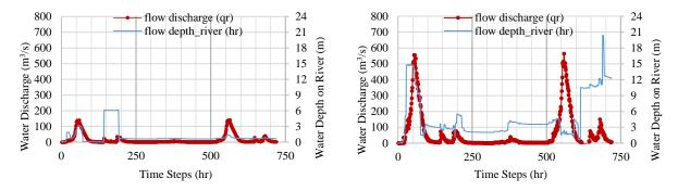
Fig. 7&8 Temporal Changes of qr and hr in Upstream & Downstream
