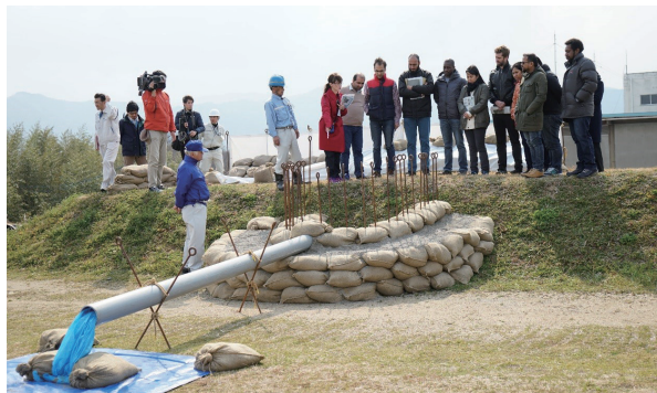
The ringing sand boil method applied to a model embankment by the officers of MLIT
