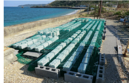
Fig-1 Outdoor Exposure Test of Concrete Specimens
