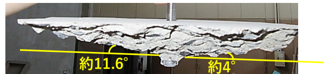
Photo-2: Typical concrete cone failure in the tensile test
