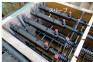
Mechanical splices used in precast concrete
