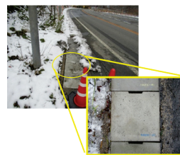
Exposure test of precast concrete made by recycled aggregate concrete Class M in severe environment
