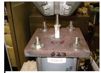
Tensile test of an adhesive anchor after immersion in alkaline solution.
