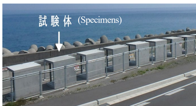
Photograph 2: Concrete specimens coated using surface-impregnation materials
