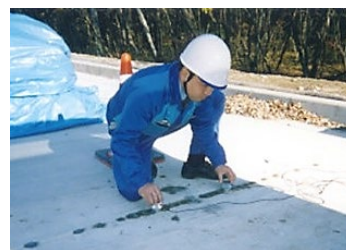
Photograph 3: Technique that uses ultrasonic wave
