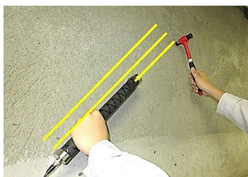
Photograph 2: Technique that uses impact elastic wave
