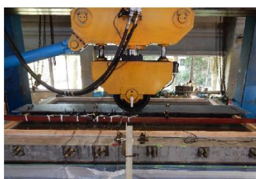
Photograph 2. Wheel running fatigue test of water-filled precast slabs joints
