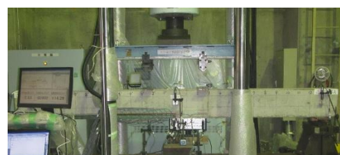
Photograph 3. Loading test applying negative bending to the bonding surface of concrete
