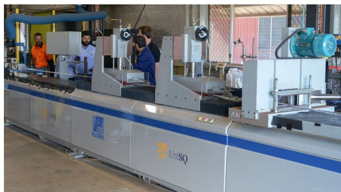
Photograph 8. Manufacturing equipment for FRP pultrusion
