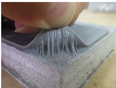
Photo. 1. Adhesive sheets for crack repair
