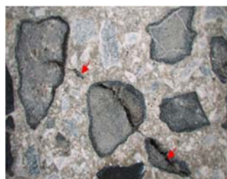
Study on the specifications for materials of concrete (observation of concrete deteriorated by ASR)
