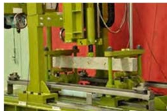
Impact loading test
